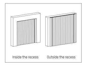
This can be done inside the recess or outside the recess. If you install the curtain rail outside the recess, it is mounted on the wall and will be placed over the window with overlap on both sides.
